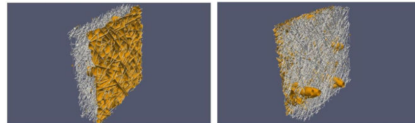
Oil interface in filter medium - inlet side
